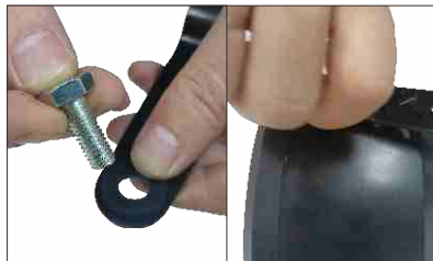
02 Remove the screw from the mounting plate shown above
