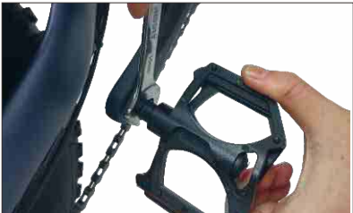
03 "R" pedal is fixed clockwise and fixed on the chain-ring
