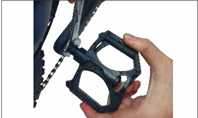
02 "L" pedal is fixed counterclockwise to the crank
