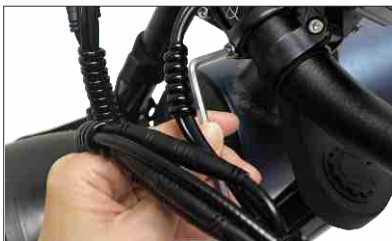
05 Mount handlebar onto stem, then replace stem cover and tighten all 4 bolts
