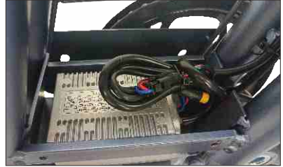
02 Controller waterproof cable
