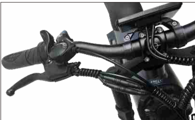
05 Connect the power-off brake handle waterproof cable
