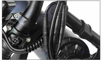
04 Connect display waterproof cable
