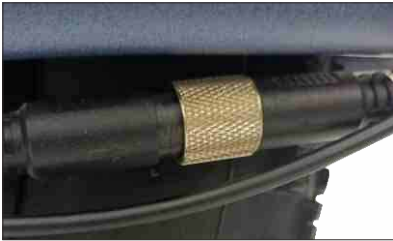
03 Connect motor waterproof cable
