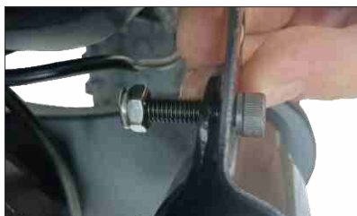
05 Remove taillight fixing screw
