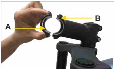
03 Tighten the side A, B screws
