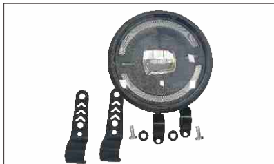
01 Remove headlights and mounting parts
