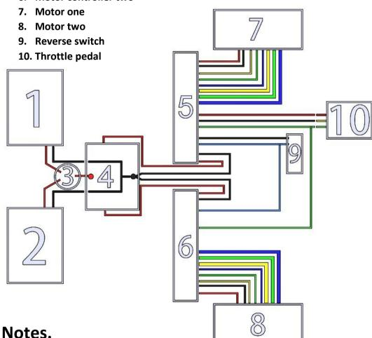
Use the 5 core and 3 core cable to join between the motor and controllers (colours don't exactly match but as long as it still connects like this that is fine.)
