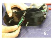
**c.** Remove the three lock nuts that attach the license plate assembly and taillight to the fender **(6)**
