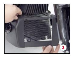
1. Remove the oil cooler cover by pulling the two lower pins from the rubber grommets on the cooler and rotate forward to allow the top to be released from tabs. (FIG 1)
