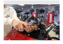
Carefully install the hardware removed in step 1 and torque them evenly to 18-20 in-lbs
