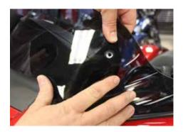
Using a 4mm Allen wrench, remove the four fasteners that hold the stock windshield to the mount brackets. NOTE: For installation on the Cross Country Tour, the Touring windshield brackets and the rubber support strips between the front and inner fairings need to be removed.
