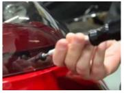
**1.** Remove the 5 stock fasteners that secure the stock windshield to the motorcycle.
