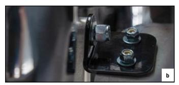
Using Hardware Bag "E", loosely install the Crash Bar Plates to the bottom of the fairing, the plates should be inside the fairing and not below it (FIG b).
