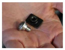
You can place low-tack tape on the back of the square nuts and bracket to help prevent them from falling into the fairing.
