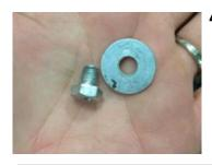
Using a 10mm wrench, remove the two mounting bolts.
