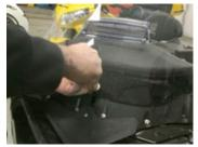
Use an 8mm wrench to loosen the windshield mounting screws and remove the stock windshield.
