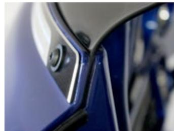
7. Secure the windshield mounting hardware, making sure that the Flare™ is resting on the mounting bosses and not on the mounting screw to avoid pinching
