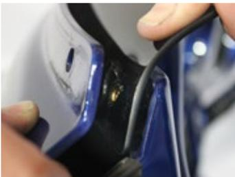
3. Guide an end of your new Klock Werks Flare™ down onto one of the outer mounting bosses
