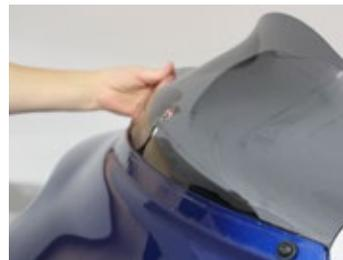
4. Guide the opposite end of the Flare™ down onto the other outer mounting boss
