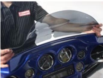
1. Remove the three windshield mounting bolts on the top of the fairing, and remove your stock windshield
