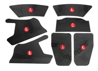
**Dynamat** components designated with a 1 must be applied before **Dynaliner** components designated with a 2.
