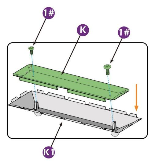
Don't fully tighten the screw 1#, It might cause problem on roofs installation.
