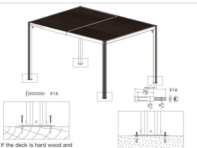
If the deck is hard wood and the depth of it is over 3 inch you can use 5/16 in. ×4 in. Structural Wood Screw to mount the pergola.
