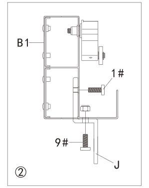
Step 3: Insert Part #J into Part #B1. Secure with 2 Bolts 1# and 2 Bolts 9# as shown.
