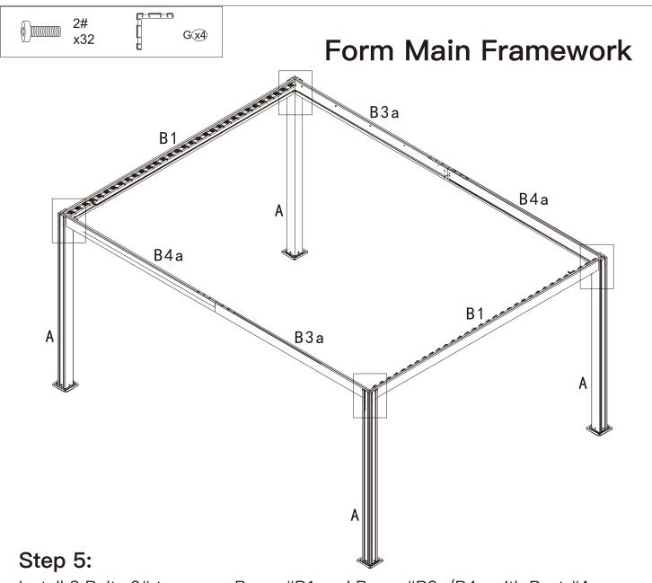
Install 8 Bolts 2# to secure Beam #B1 and Beam #B3a/B4a with Post #A, Then install Part #G into Corner Post #A as shown.
