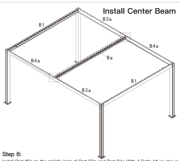
Install Part #Ba to the middle joint of Part B3a and Part B4a With 4 Bolts 1# as shown. Repeat the above procedures to assemble another side.
