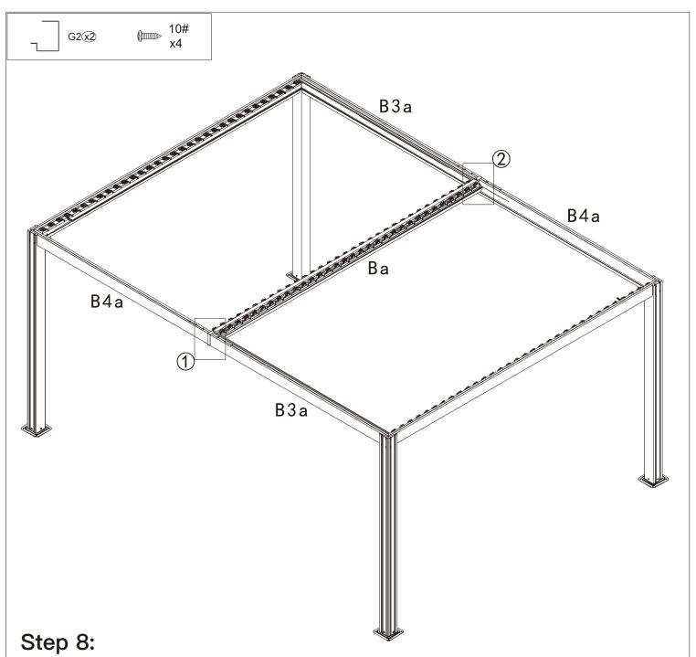
Install Part #G2 at the joint of Part #B3a and Part #B4a with 2 bolts 10# as shown. Repeat the above procedures to assemble another side.
