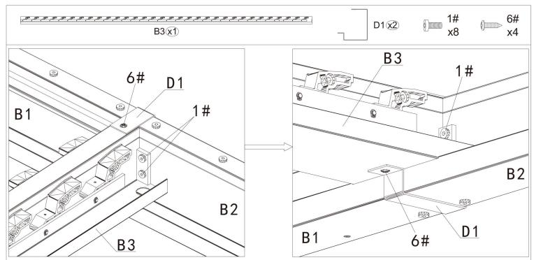
**Step 7:** Fix Part D1 to Part B3 and Part B2 with screw 6# and 1# as shown above. After the completion of this step, each part is as shown in the following figure.
