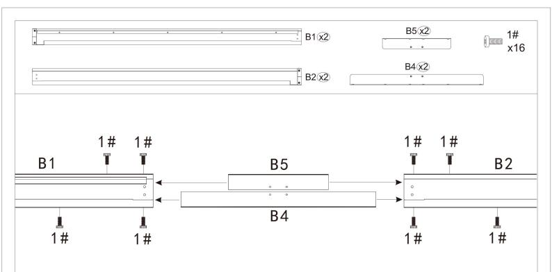
Step 2: Place Part B5 and Part B4 into Part B1 and B2 with screws 1# as shown above.
