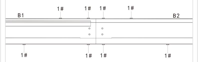
Step 3: Connect Part B1 and Part B2 with screws 1# as shown.
