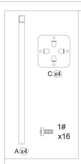
**Step 1:** Connect Part A and Part C with screws 1# as shown.
