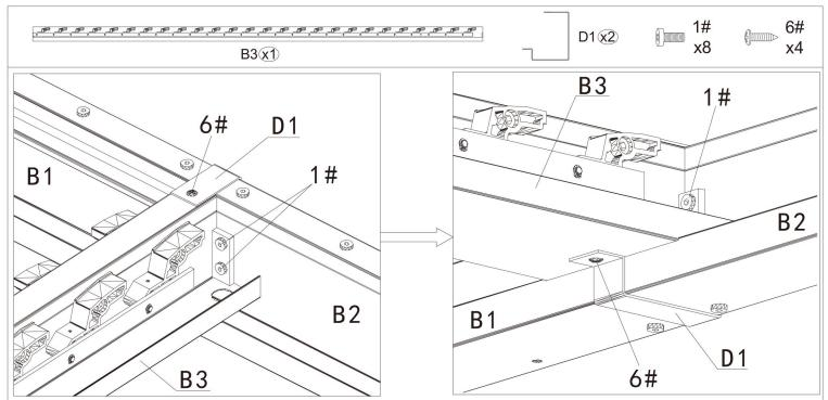
Step 7: Fix Part D1 to Part B3 and Part B2 with screw 6# and 1# as shown above. After the completion of this step, each part is as shown in the following figure.
