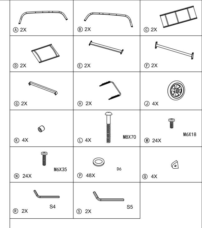
Friendly Tip: Please do not completely tighten the screws during assembly. After all the screws are assembled in place, tighten them together. Remember to wear gloves.
