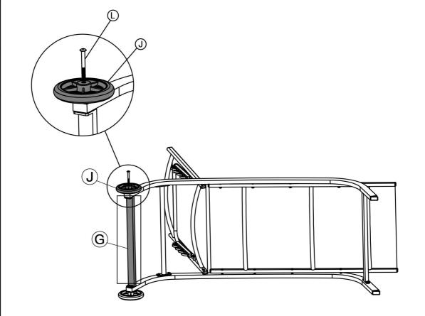
Step 7: Tighten all the screws and turn the chair around.
