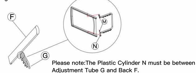
Step 3: Connect Back F to Main Seat Frame A using Bolts L (M6×35) as shown in diagram.
