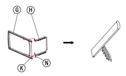
Assemble backrest and adjustable gear to the seat Part B with screws Part R.
