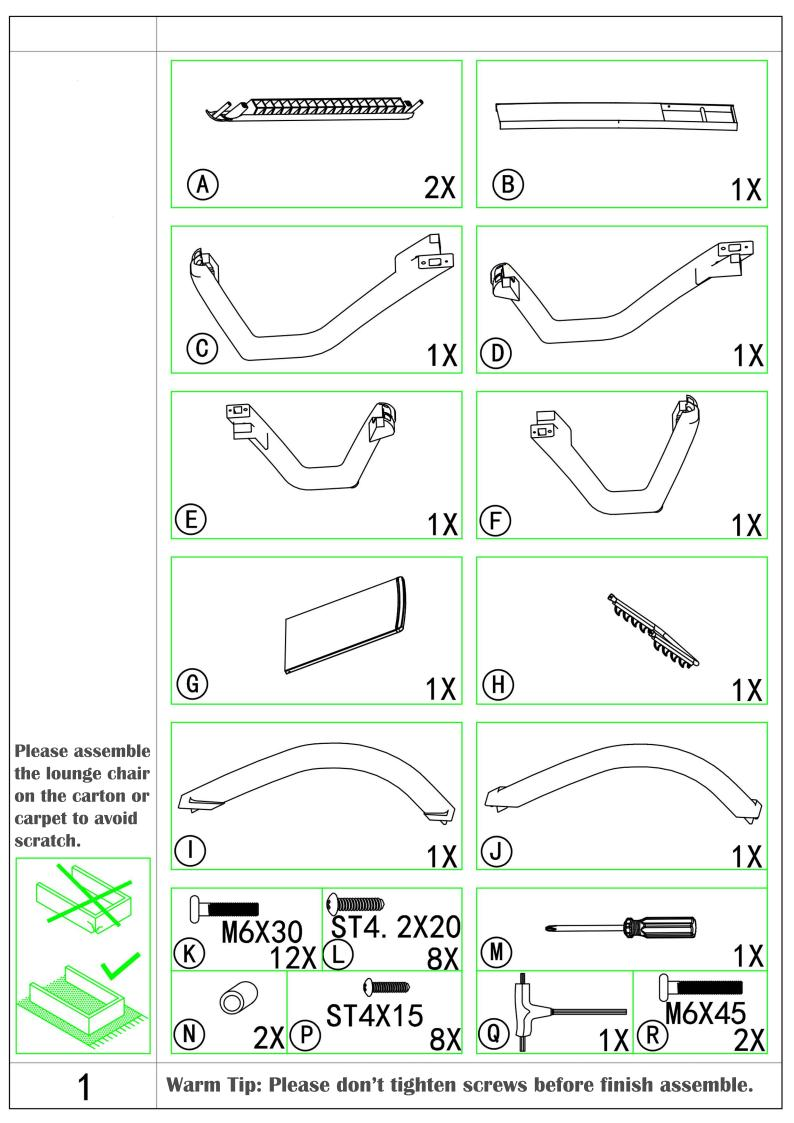
(K)**Assemble four** (B) legs Part C,Part **D,Part F and** Part E to the (D)seat Part B with srews Part K. **Assemble Part A** to the seat Part B, then assemble **Armrest Part I** and Part J to the seat Part B. Then use screws **Part L and Part** P to lock the legs. Tighten all srews before using.
