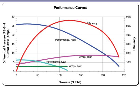
These performance curves are a result of in-lab testing using 3" suction line, actual performance may vary based on manufacturing tolerances and application.
