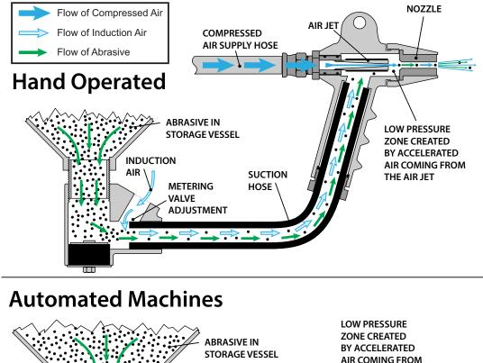
ABRASIVE IN STORAGE VESSEL INDUCTION AIR METERING AJUSTMENT COMPRESSED AIR SUPPLY HOSE Suction blast systems work by drawing abrasive to the nozzle using suction instead of pushing it through a blast hose with compressed air.
