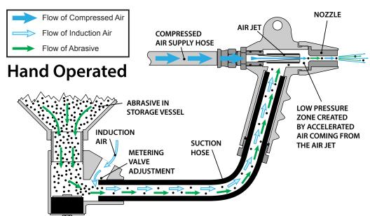
Suction blast systems work by drawing abrasive to the nozzle using suction instead of pushing it through a blast hose with compressed air.
