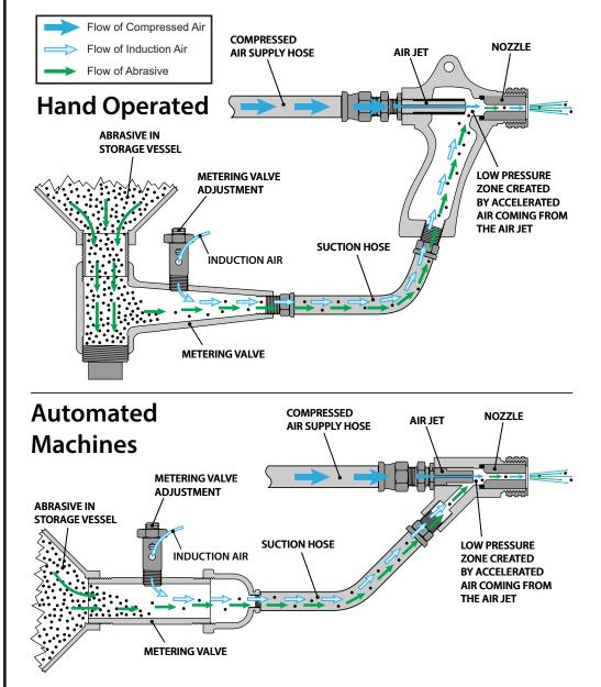
Suction blast systems work by drawing abrasive to the nozzle using suction instead of pushing it through a blast hose with compressed air.
