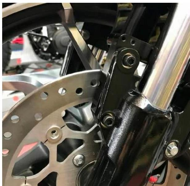
5. While pushing lightly down on the front tip of fender, tighten the (4) 5/16 x 1/2” bolts paying attention while tightening to the rear of fender staying centered over tire.
