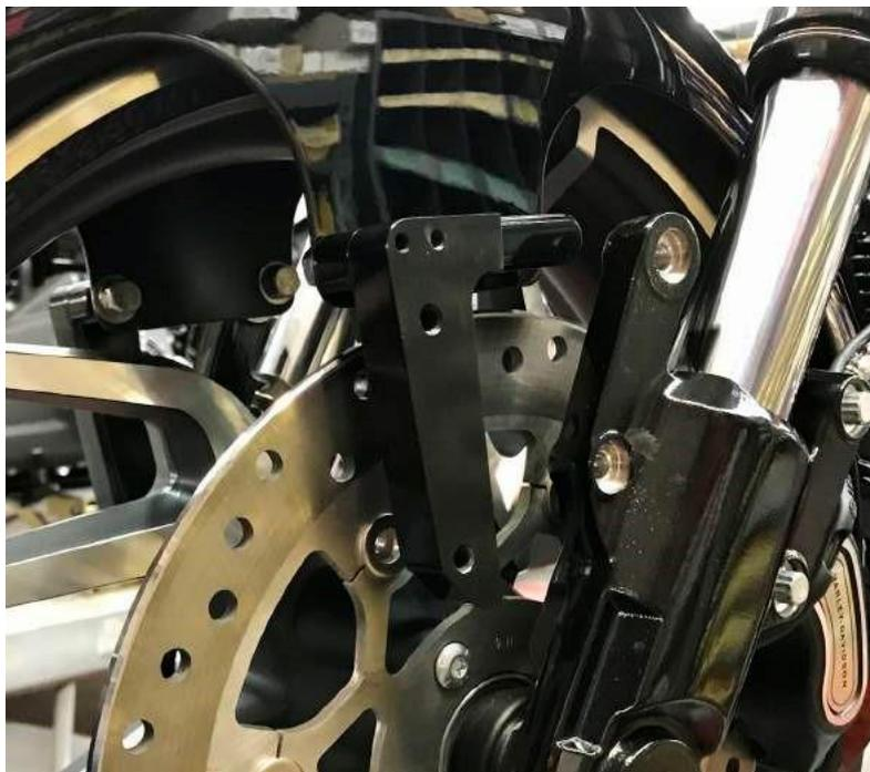
3. Slide fender in place over tire & repeat step #2 only this time with the bracket marked “L” on the left side (Fig # 4) Again, **BLUE LOCTITE®** and finger tighten only.
