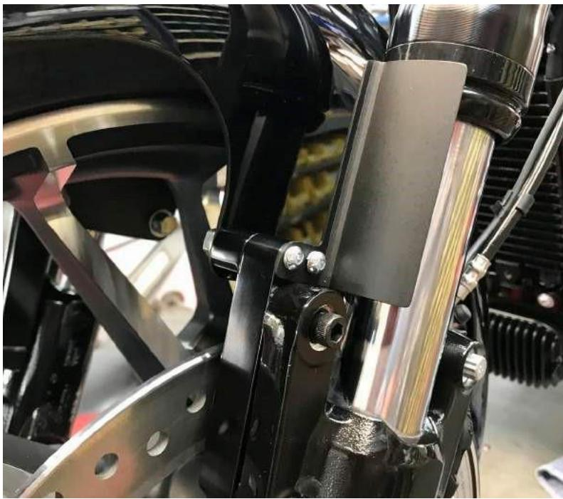
6. Install debris guards on right & left sides. Check fender fastener torque & gently turn wheel from side to side for clearance. Squeeze front brake & depress fork checking for paper travel clearance. (Fig #6)
