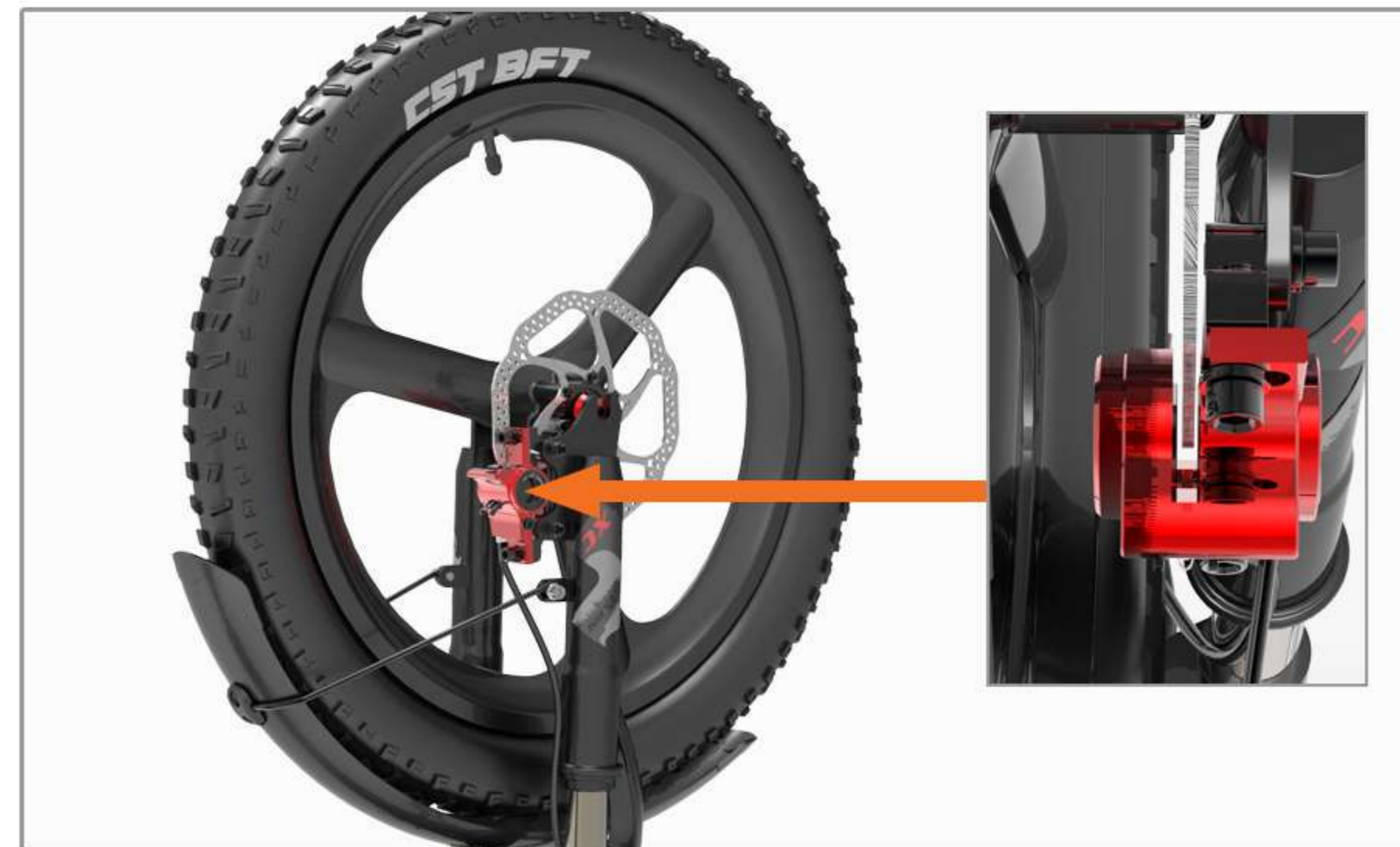
05 Put the wheel in the front fork Disc brake disc alignment clamp card slot
