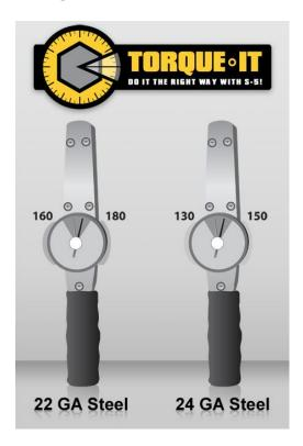
When relying upon published load values, setscrew tension should be periodically verified using a calibrated torque wrench between 160 and 180 inch-pounds (not foot pounds) (18-20 Nm) when used on 22 gauge steel or between 130 and 150 inch-pounds (15-17 Nm) on 24 gauge steel.
