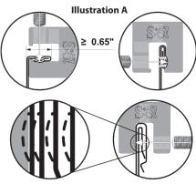
(Top) S-5-U clamp on both vertical and horizontal seams. (Bottom) S-5-S on a snap together seam with blow up illustrating deformation of seam as setscrew is tightened **For horizontal seams equal to or greater than .65" use the** S-5-U in its horizontal orientation.
