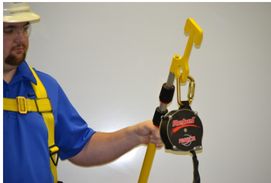
Figure 7 - SRL Attached to Anchor via Carabiner
