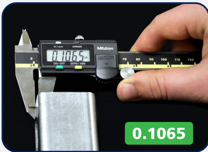
UNISTRUT® P1000 PG 12 gauge strut - typical results
