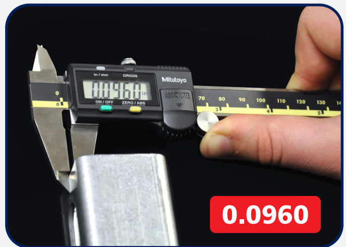
Competitor 1 "12 gauge strut" - 3.5% below minimum
