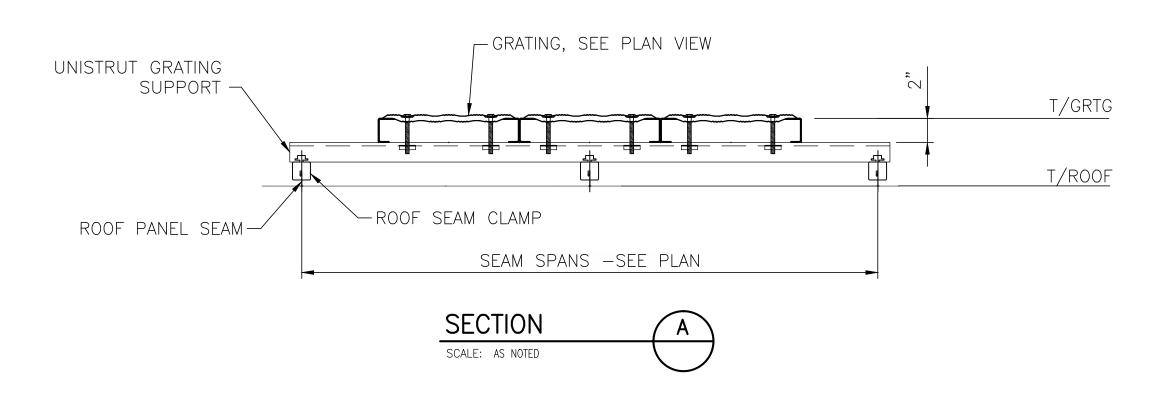
STANDARD UNISTRUT WALKWAY DETAIL PARALLEL TO STANDING SEAMS W/ NO RAIL
