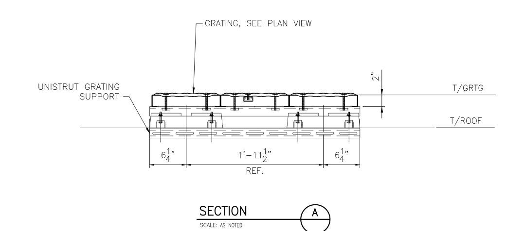
STANDARD UNISTRUT WALKWAY PLAN ON FLAT ROOF W/ NO RAILS PART NO. RWOHRFRWB (RUBBER BASES) SCALE: 1-1/2"=1'-0" (WHEN PLOTTED FULL SIZE)
