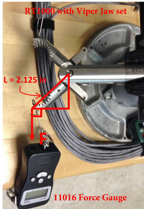
Force Test Setup
