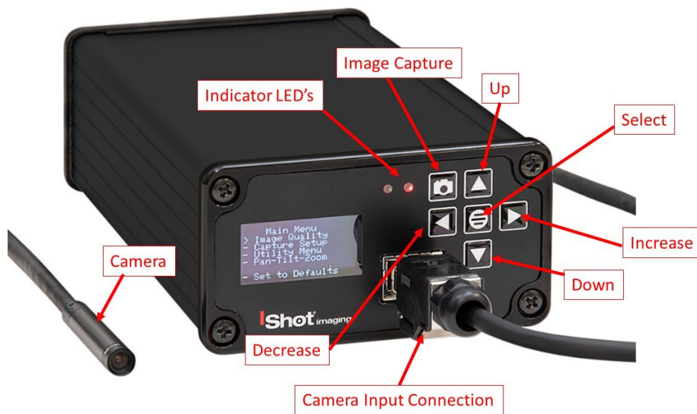
Figure 4 Labeled Front of CCU
