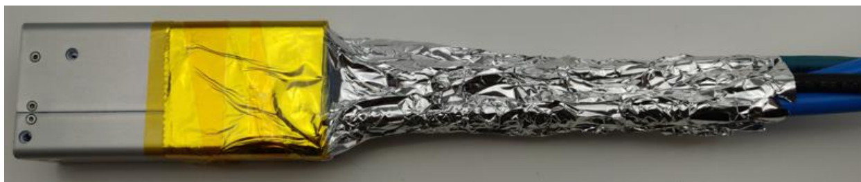
Fig. 3.3. Aluminium foil wrapped around camera housing, cables and hoses.
