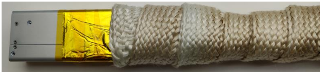
Fig. 3.7. Thermosleeve B wrapped around the cables and hoses (effectively two additional layers).
