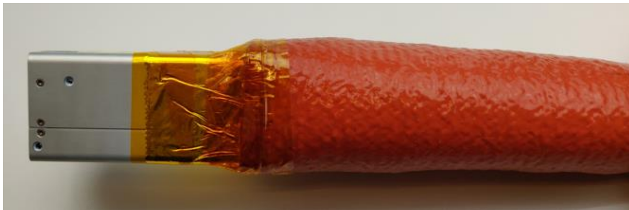
Fig. 3.8. Pyrojacket pulled over the cables and hoses and sealed to camera housing with Kapton tape.
