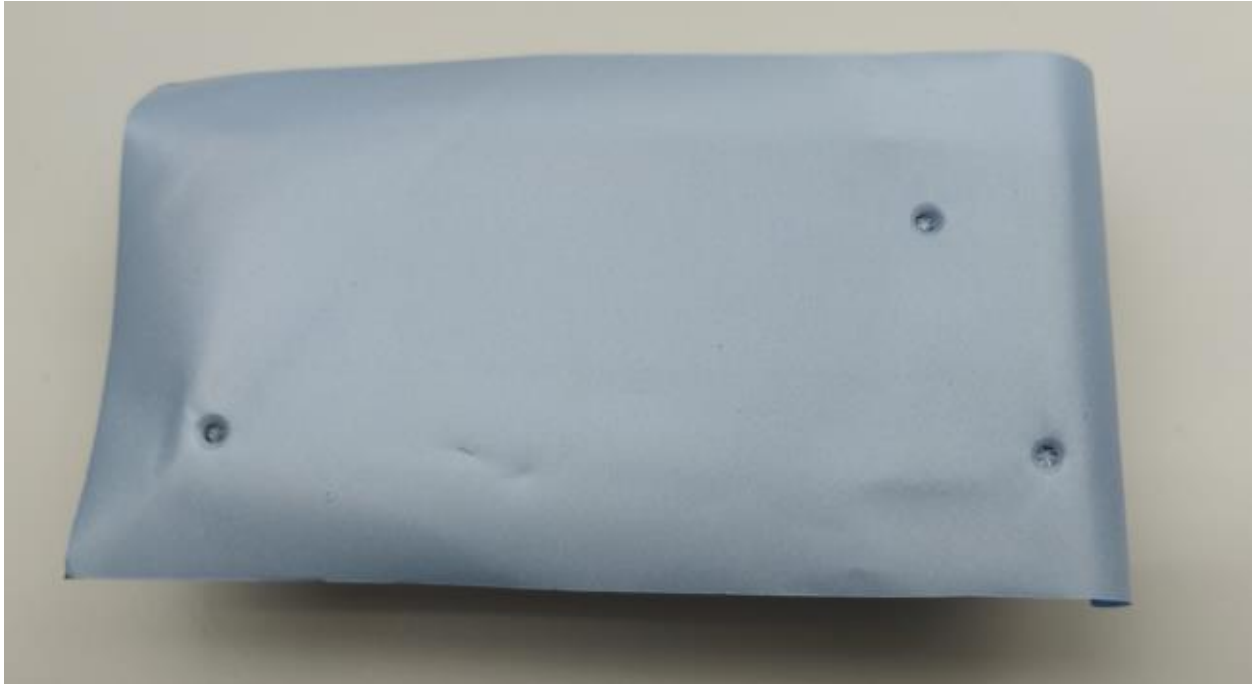
Fig. 2.4. Place the thermally conductive sheet over the camera and mark the locations of the threads.
