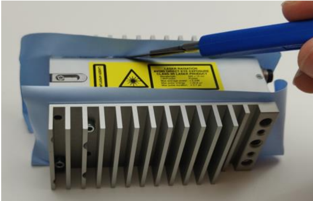
Fig. 2.8. Remove excess sheet, if applicable.
