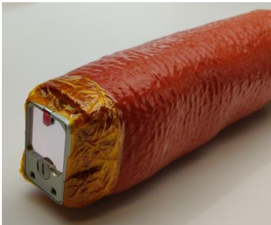
Fig. 3.5. Interface between camera housing and outermost protective sleeve sealed with Kapton tape.
