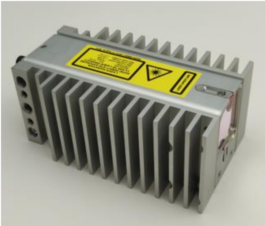
Fig. 2.9. Heat sinks successfully mounted.
