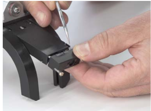
Figure 4 - Align fixed and moveable pins. Note moveable pins align with slots (see pointer)
