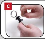
Remove the slide lock screw from the slide handle.
