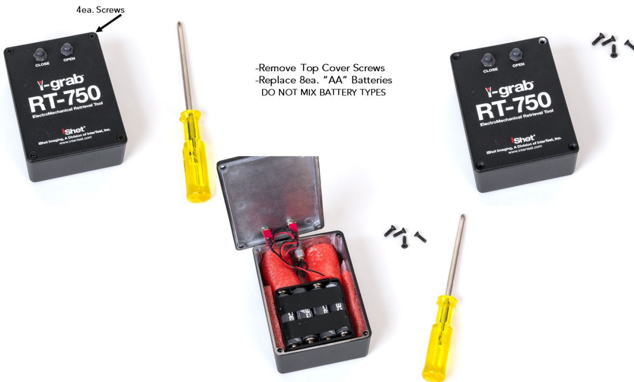
Figure 11 Battery Replacement
