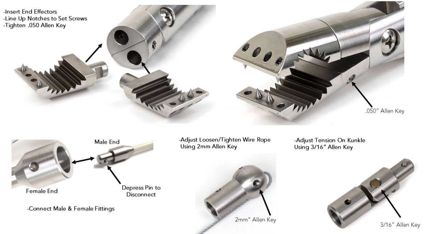
Figure 9 Tool Connections & Adjustments
