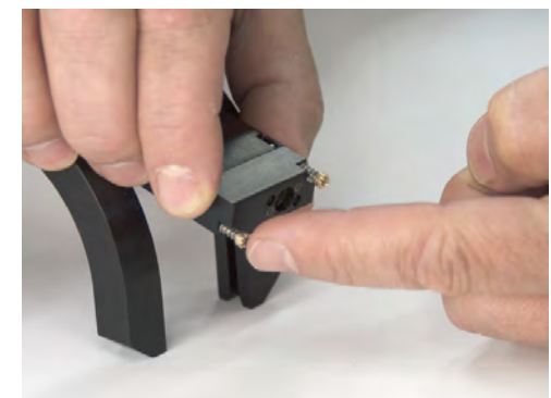
Figure 6 & 7 - Push and rotate pins clockwise 90° to engage counter clockwise 90° to disengage
