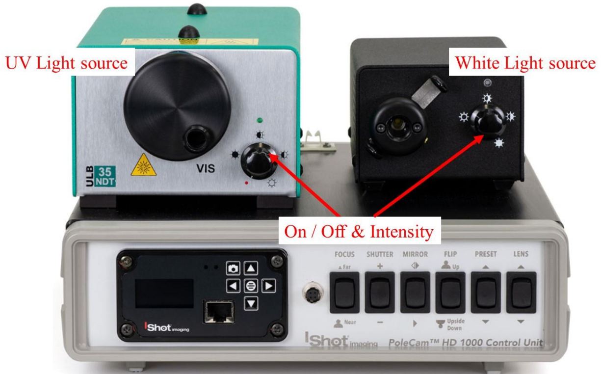
Figure 6 ON/OFF Controls Light Sources
