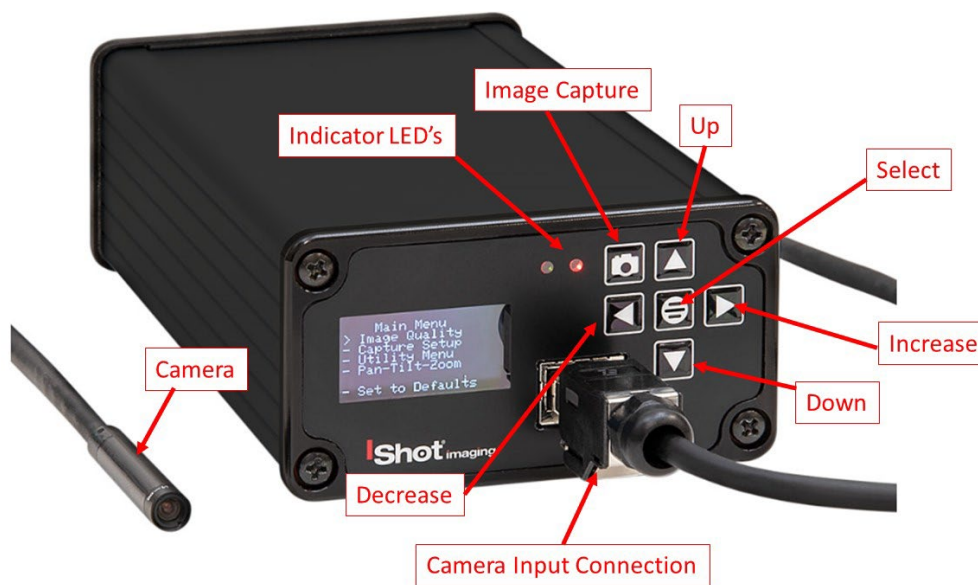
Figure 7 Labeled Front of CCU
