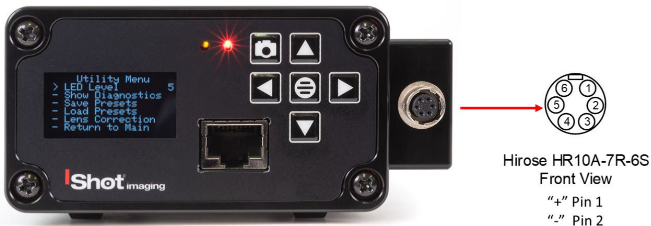
Figure 12 LED Version CCU Pin Out
