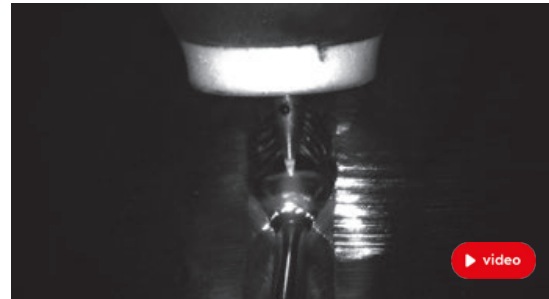
NARROW GROOVE WELDING (SAKKY FINLAND)
