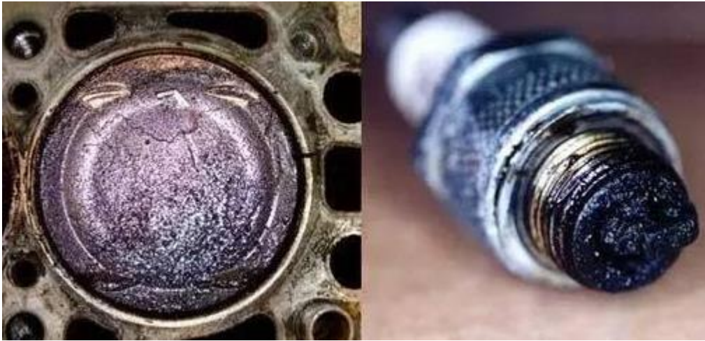
Piston and spark plug carbon
