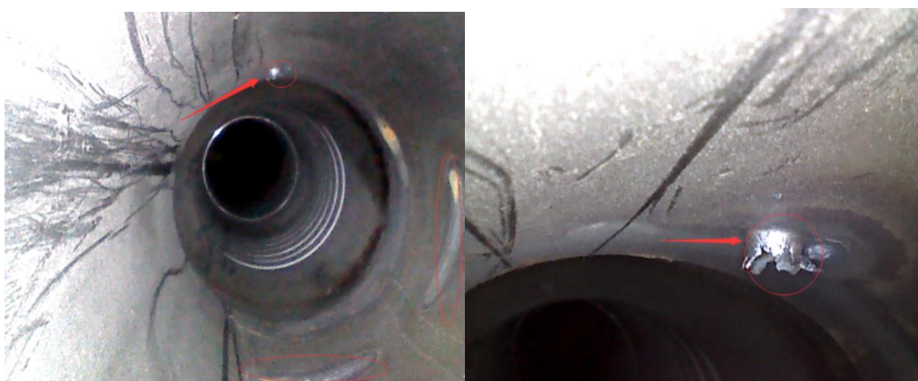
The inside flaw of the exhaust pipe
