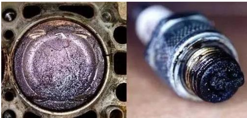
Piston and spark plug carbon
