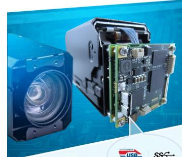
The new compact 4K to USB3 interface board is a highperformance USB3 SuperSpeed video capture module.
