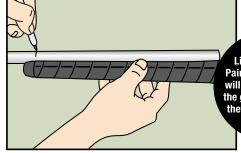
**3.** Hold the JumboMax Grip next to the shaft to determine how much of the shaft will be covered by the grip. Mark one inch from end of the grip with china marker.
