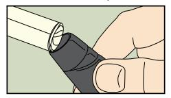
**8.** Remove the tee. Squeeze open end of the grip and start it over the butt end of the shaft. With both hands, push firmly while twisting to install the grip as far as it will go. If it will not go easily, pull off immediately, re-wet everything with solvent & start over.
