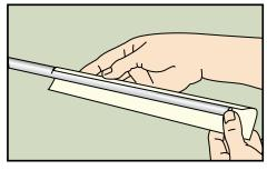
**4.** Apply double-sided grip tape beginning at your mark and leaving an inch overlap at the shaft butt.
