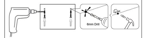
Use a electric drill to punch four 6mm holes at the marked spots, and then apply wall anchors with hammer. (6mm drill bit, drilling depth in 5 cm)
