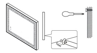
Use a screwdriver to screw the screws into the wall anchors. Leave a distance of 7 mm from the wall.
