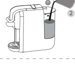
Before using for the first time or after long pauses (e.g. holidays) the machine may be difficult to pump water, this short procedure can help pump to self priming by using the pipe to fill water into the circuit manually prior to turn on the machine for first refill.
