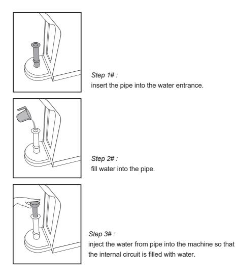
After above steps, the machine will be able to pump water out normally.
